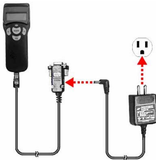
Figure 3: Connecting the Power Adapter
