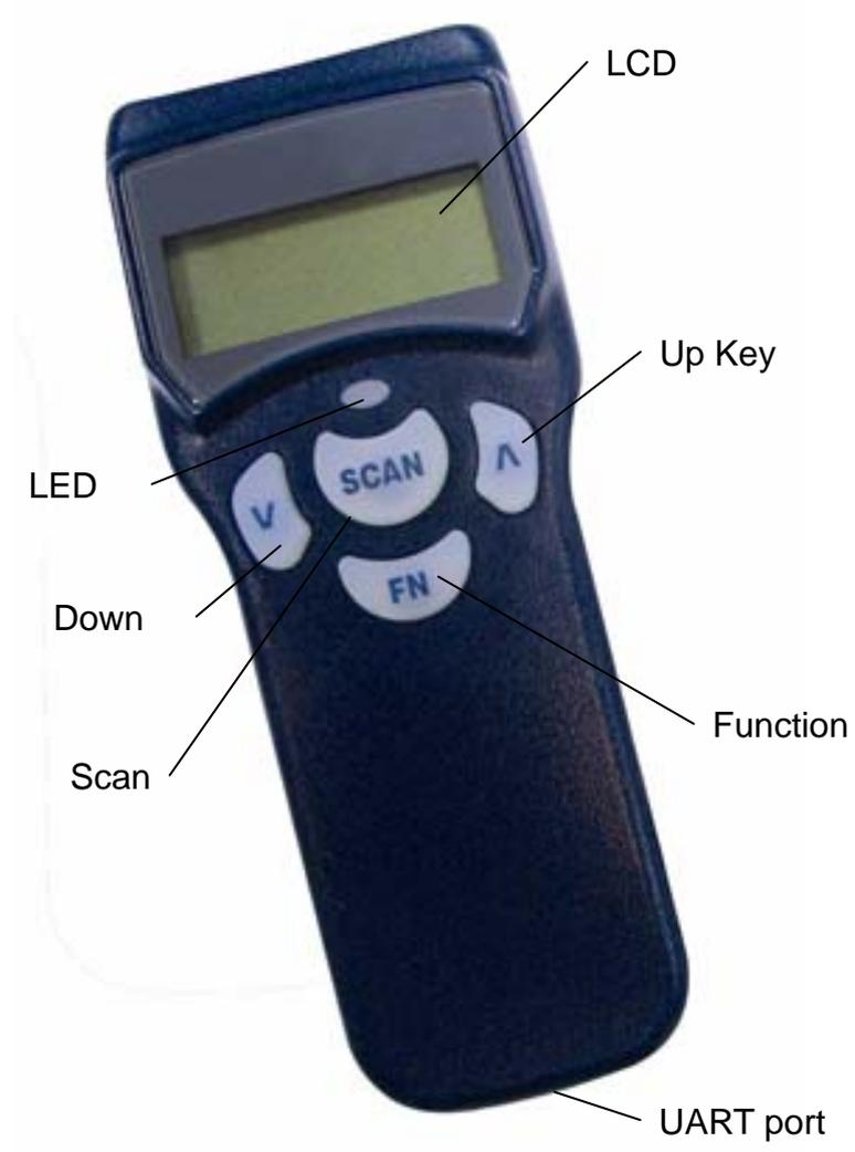
**Figure 1: Pocket-Sized Personal Data Collector**
