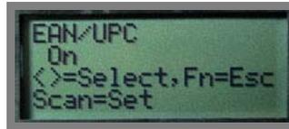
Figure 12: Barcode Setup
