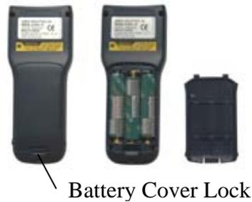
**Figure 2: Inserting Batteries**
